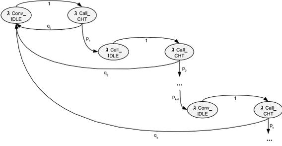
**Figure 7. n-state (On/Off-Model) (semi-) markov model**
