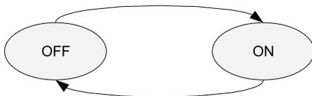
**Figure 1. two state (On-/Off-Model) (semi-) markov model**
